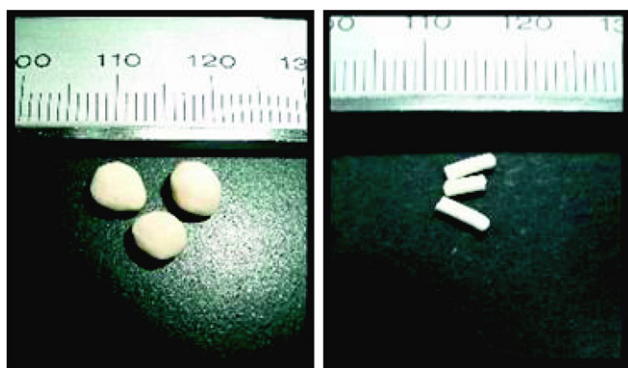
Fig. 3 Pictures of new adsorbent ( left ) and common 1/16 pellet adsorbent ( right )
